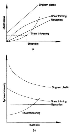
Figure 1.19 Flow curves for time-independent fluids (a) Shear stress against shear rate (b) Apparent viscosity against shear rate
