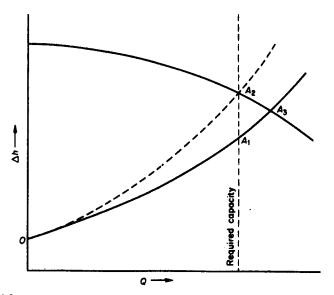
Figure 4.8 Effect of adding a safety factor to the system total head against capacity curve
