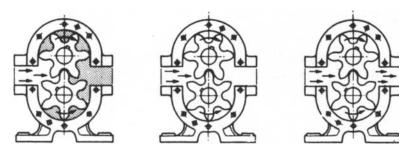
Figure 4.11 Operation of an external gear pump
