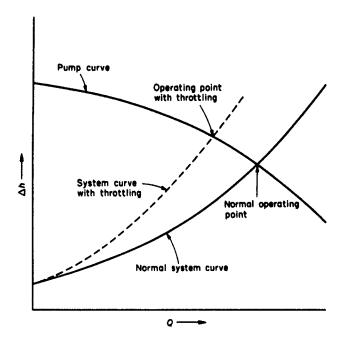
Figure 4.7 Effect of throttling the discharge valve on the operating point of a centrifugal pump
