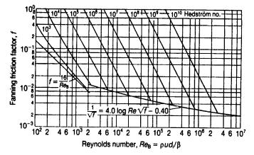
Figure 3.10 Friction factor chart for laminar flow of Bingham plastic materials. (See Friction Factor Charts on page 349.)
