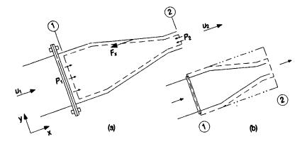
Figure 1.9 Forces acting on a nozzle inclined at angle  $\theta$  to the horizontal (a) Internal control volume. (b) Two possible external control volumes
