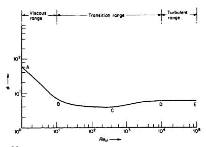
Figure 5.8 Power curve for the standard tank configuration
