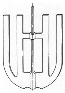
Figure 5.6 Gate type anchor agitator
