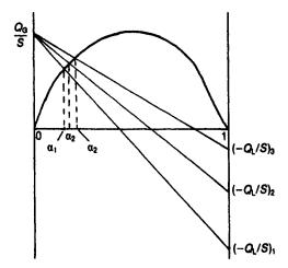
Figure 7.9 Wallis plot for cocurrent flow
