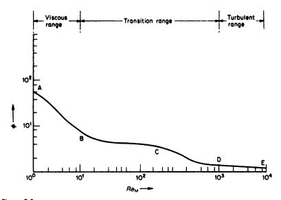
Figure 5.9 Power curve for the standard tank configuration without baffles
