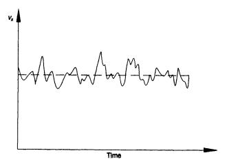
Figure 1.22 Variation of the velocity component vx in turbulent flow
