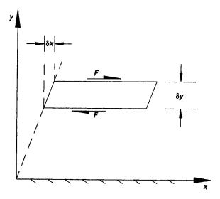
Figure 1.11 Shearing of an element of material
