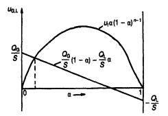
Figure 7.8 Wallis plot for flow in a bubble column
