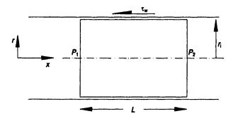
Figure 1.15 An element of fluid extending over the whole of the pipe cross section
