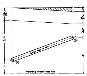
Figure 1.5 Diagrammatic representation of heads in a liquid flowing through a pipe
