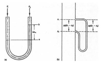
Figure 8.1 U-tube manometer
