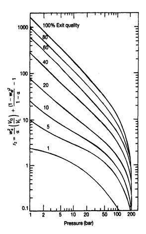
Figure 7.17 Factor r<sub>2</sub> as a function of absolute pressure Source: R. C. Martinelli and D. B. Nelson, Transactions of ASME, 70, No. 6, pp. 695-702 (1948)
