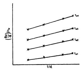
Figure 3.12 Plot of apparent fluidity against 1/d, to determine the slip velocity (Mooney's method)
