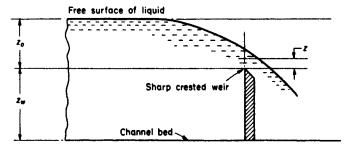
Figure 8.8 Flow of liquid over a sharp—crested weir
