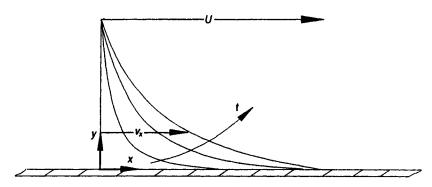
Figure 10.2 Fluid velocity as a function of time and distance from the plate
