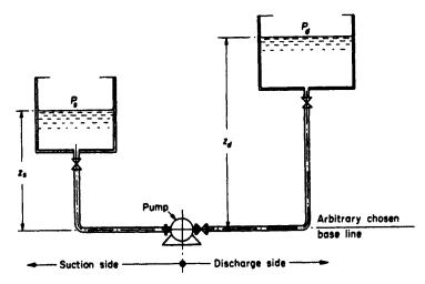
Figure 4.1 Typical pumping system
