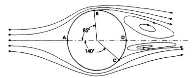
Figure 9.1 Streamlines for flow around a sphere Upper half: intermediate Rep giving a laminar boundary layer
