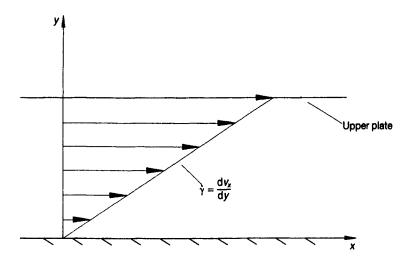
Figure 1.12 Shearing of a fluid showing the velocity gradient
