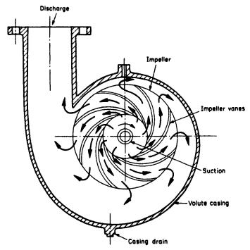
Figure 4.2 Volute centrifugal pump casing design
