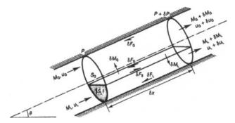
Figure 7.6 Element of two-phase flow
