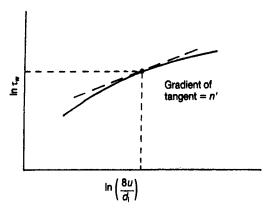
Figure 3.6 Logarithmic plot of wall shear stress against flow characteristic: the gradient at a point defines n'
