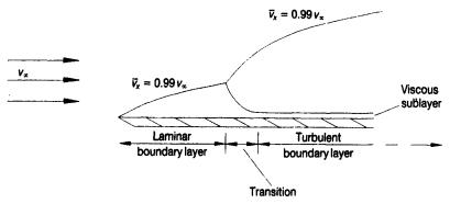
Figure 1.25 Laminar and turbulent boundary layers over a flat plate
