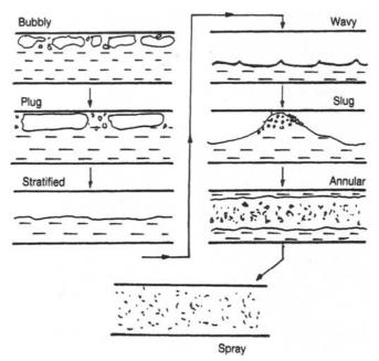
Figure 7.2 Flow regimes in horizontal gas-liquid flow
