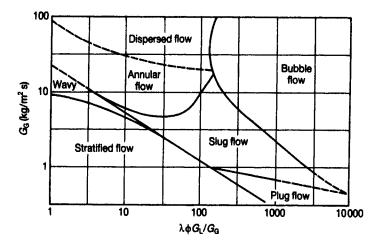
Figure 7.4 Flow regime map for horizontal gas-liquid flow Source: O. Baker, Oil and Gas Journal 53, pp. 185-95 (26 July, 1954)
