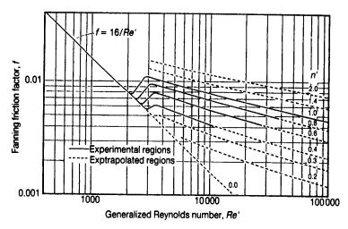
Figure 3.8 Friction factor chart for purely viscous non-Newtonian fluids. (See Friction Factor Charts on page 349.)
