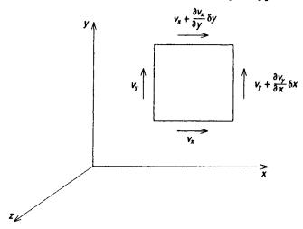
Figure A.1 Velocity components for a two-dimensional flow
