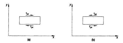
Figure 1.16 Sian conventions for stress (a) Positive sign convention (b) Negative sign convention
