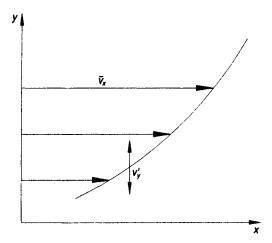
Figure 1.23 Velocity fluctuation in the y-direction across the gradient of the mean velocity
