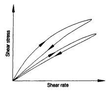
Figure 1.21 Flow curves for a thixotropic fluid
