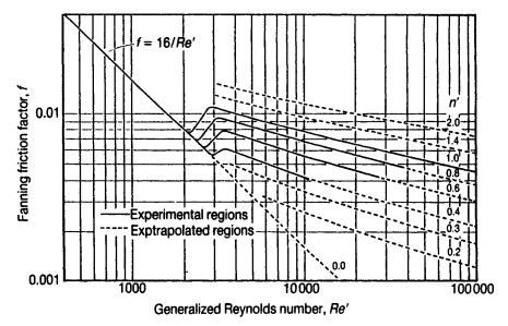
Friction factor chart for purely viscous non-Newtonian fluids
