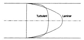
Figure 1.24 Comparison of the time-averaged velocity profile for turbulent flow and the profile for laminar flow at the same volumetric flow rate
