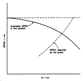
Figure 4.5 Available and required net positive suction heads against capacity in a pumping system
