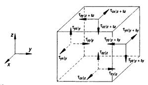
Figure 1.18 Negative sign convention for stress components. The diagram shows the directions in which components are taken as positive. The components acting on the faces normal to the x-axis have been omitted for clarity
