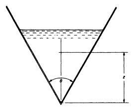
Figure 8.9 Cross-sectional flow area in a V-notch weir
