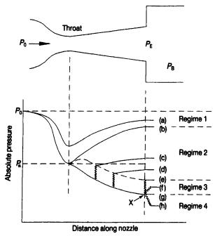
Figure 6.2 Pressure profiles for compressible flow through a convergent-divergent nozzle
