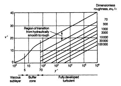
Figure 2.5 Universal velocity profile for turbulent flow Source: N. Scholtz, VDI-Beriche 6, 7-12 (1955)
